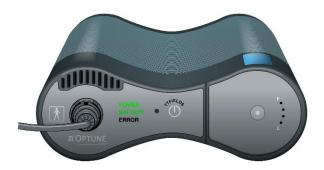
If a power supply, connected to the mains, is plugged into the device, the device will run off of the power supply and the "Battery" indicator will not illuminate.
