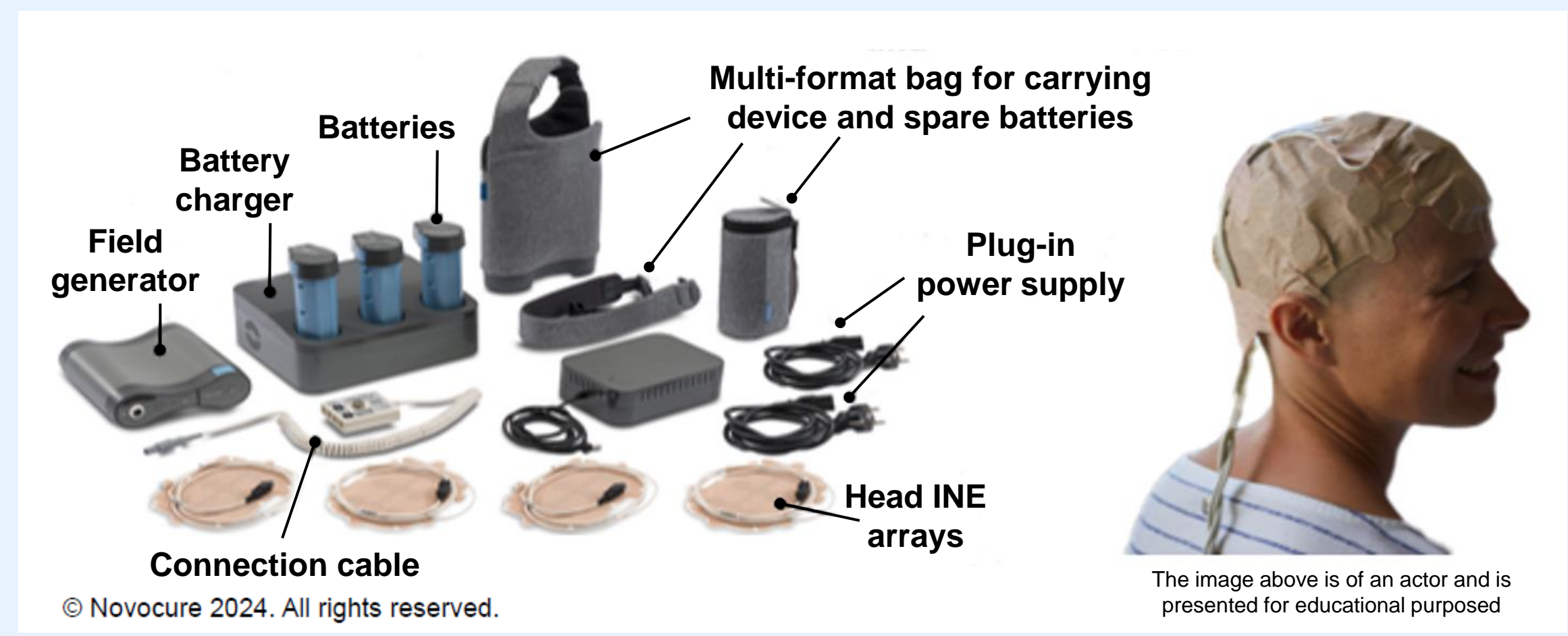
Figure 1. NovoTTF-100A system for use in glioblastoma 5–7
