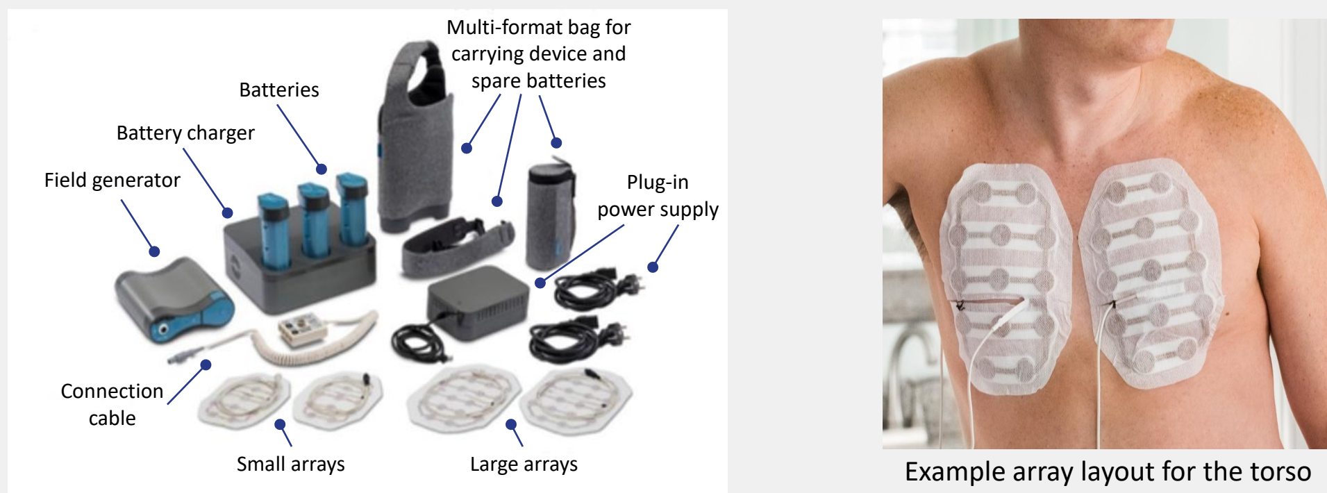
Figure 1. The TTFields device components and example array layout
