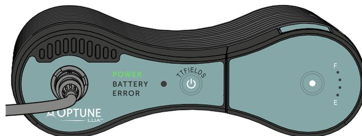
NOTE: If a charged battery is installed (and no power supply is connected), the green "BATTERY" indicator illuminates. If the device is connected to the power supply, it will be operated from the power supply and the "BATTERY" indicator will turn off.
