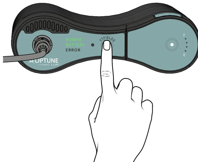
The "TTFIELDS" indicator, above the TTFIELDS ON/OFF button, should illuminate in blue and stay on while the treatment is ON.
