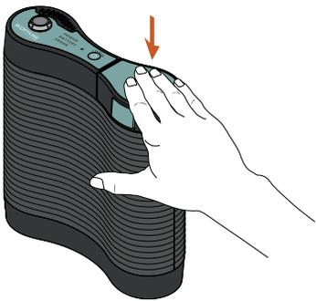
**Gently press down to lock the battery in place.**
